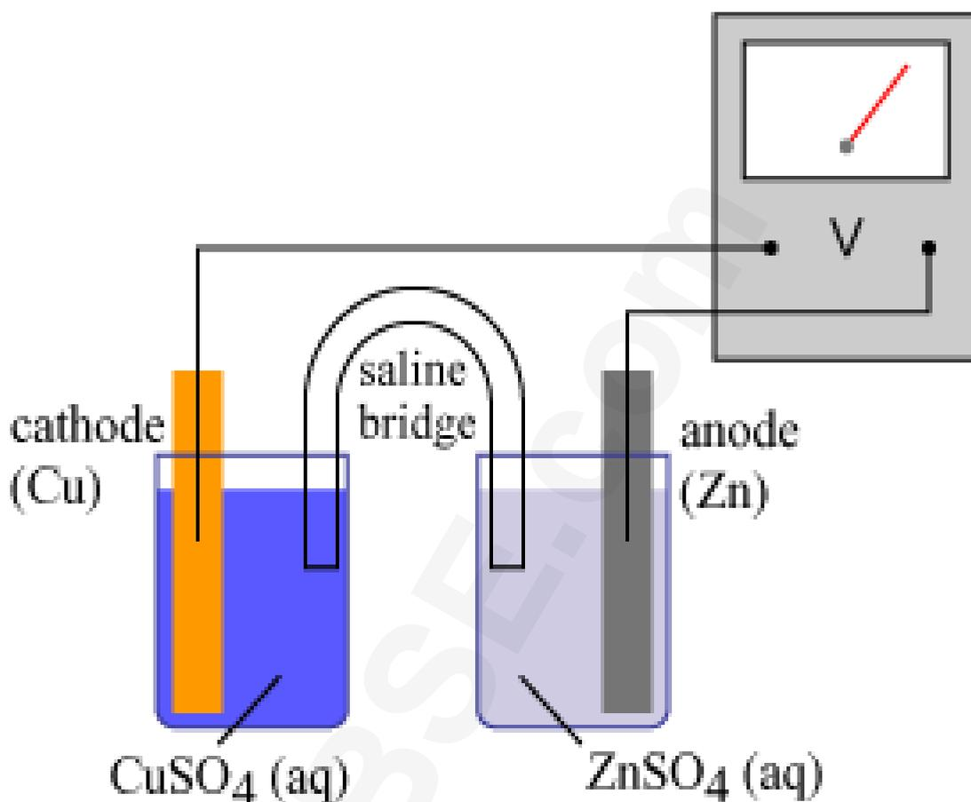
When an external circuit is connected, the chemical equation for the zinc side (anode) half cell is:
